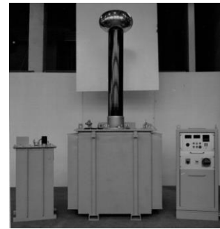
Conventional Test System 300kV
