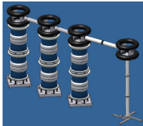
< Test configuration 560kV with 6 reactors DSH6W
